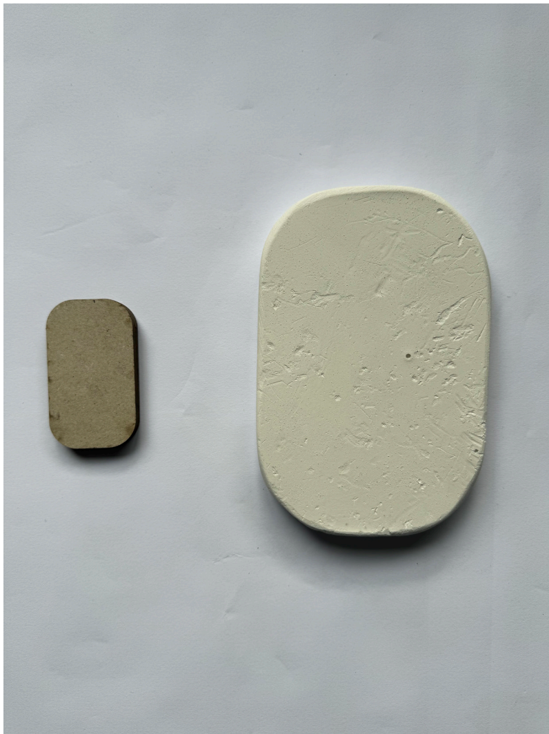
Cutting a floor from the RAvB building—Models: left, wood-laser cut; right, casted plaster.
