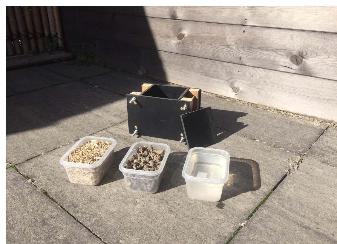
HEMPCLAY INGREDIENTS : 1 PART WATER - 2 PARTS SEACLAY - 3 PARTS HEMPSHIVES (30-50MM)
