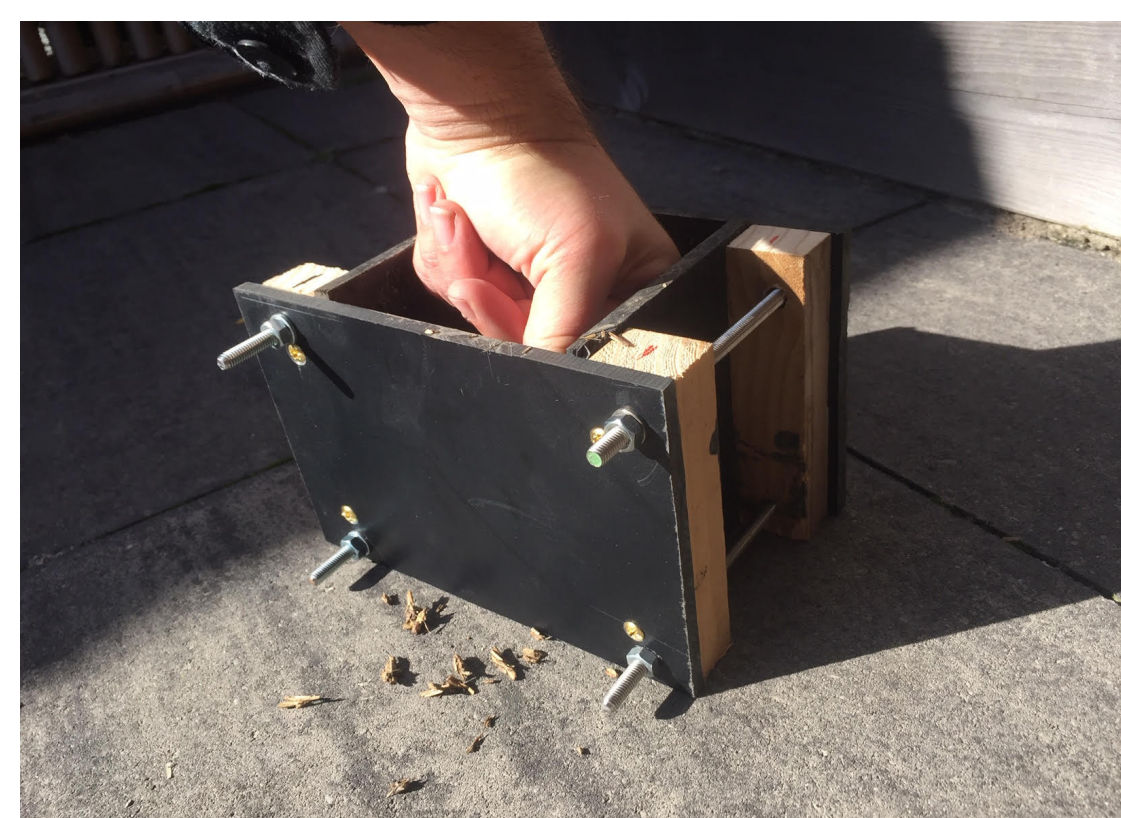
POUR THE MIXTURE IN THE MOULD AND PUT THE TOP ON. HANDPRESSING GIVES A QUICK AND GOOD RESULT
