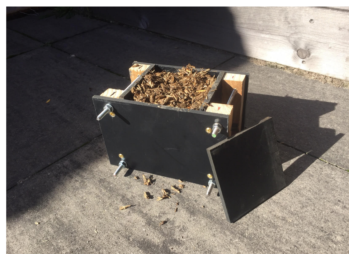
MIX WATER AND CLAY TO A MUDDY SUBSTANCE. ADD HEMPSHIVES IN SMALL PORTIONS BY KEEPING AN EYE ON THE STICKYNESS OF THE MIXTURE
