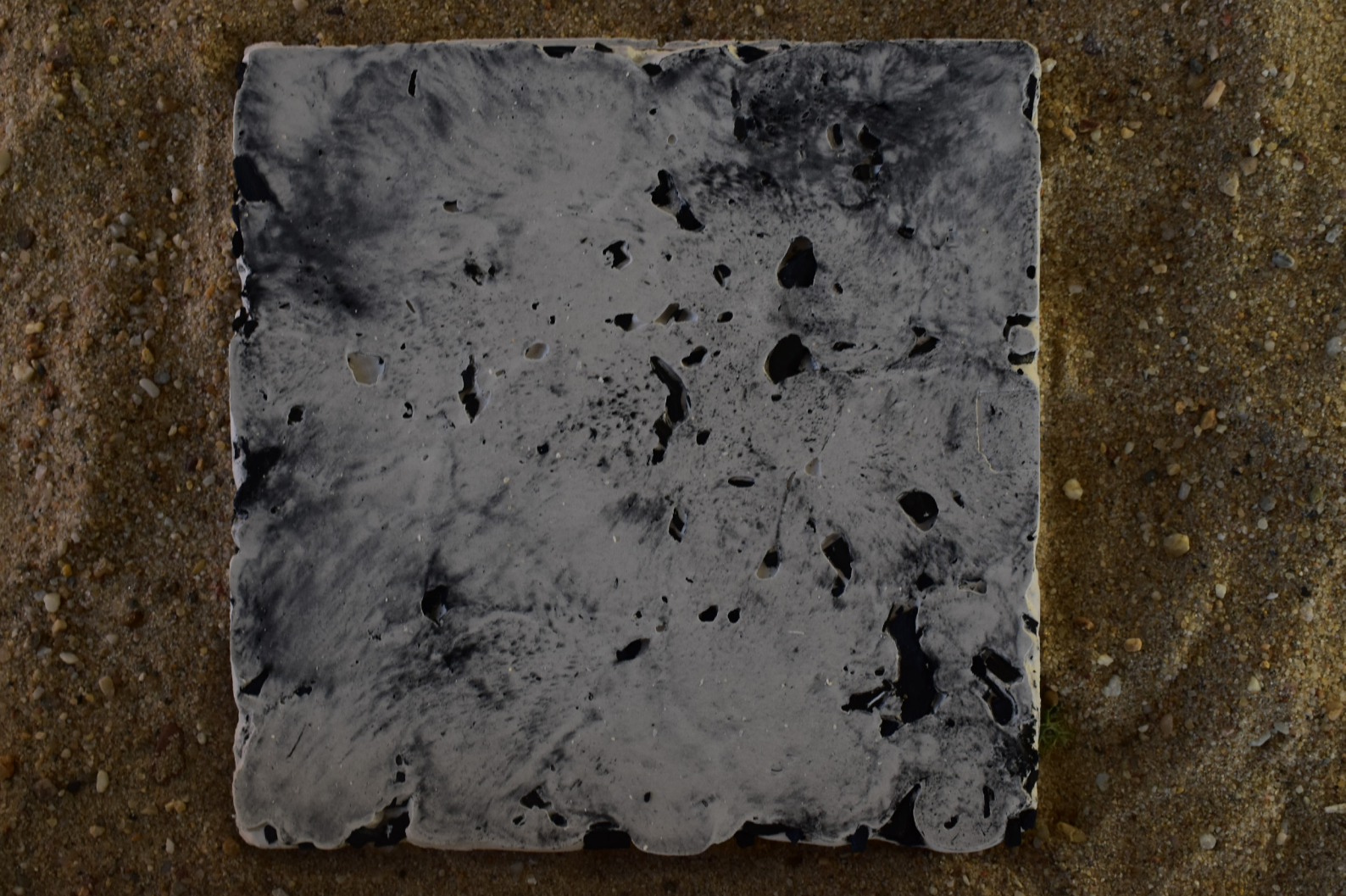
sample of concrete (here: plaster) with shell dust and fragments (here: coal)
